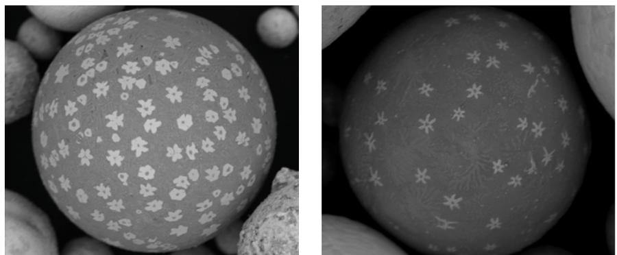
Figure 3 - Bright coloured tungsten rich features in Fe-WC cermet powder material
