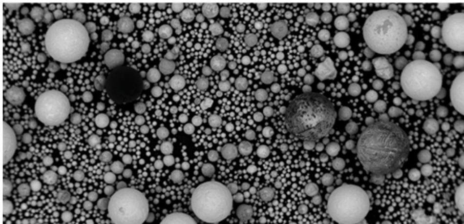
Figure 1 - Early trial of spheroidised WC showing particles with differing elemental composition
